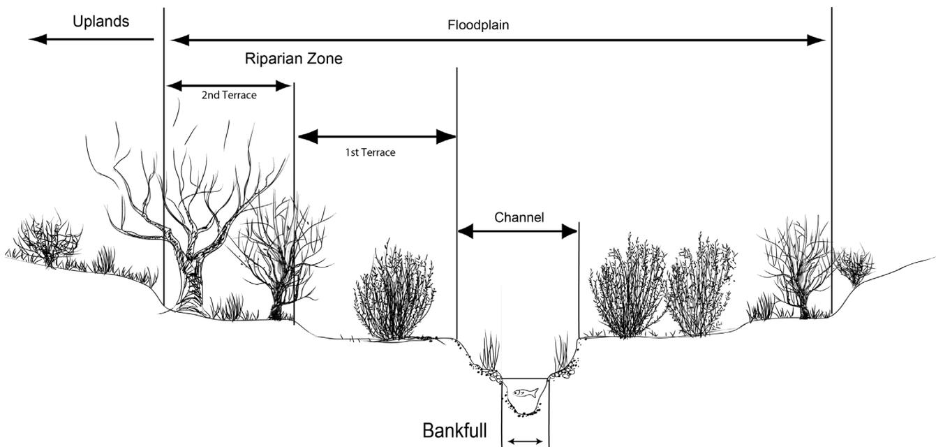
**Figure 11:** Idealized cross section of a downcut stream and associated floodplain in the American Southwest. Areas of the floodplain outside of the scour zone are flooded only during rare and high flow events. In entrenched streams, the second terrace represents the pre-entrenched floodplain. The edge of the first terrace close to the stream channel marks the inside edge of the riparian zone as used in this protocol, and the riparian transect should be put there. *Credit: Heidi Snell.*
