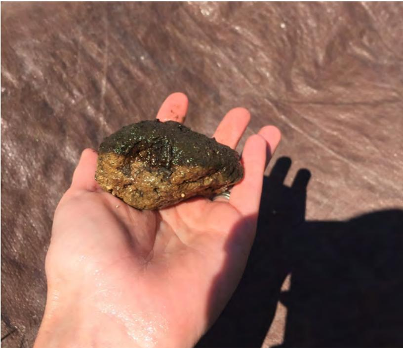
**Figure 23:** Cobble Embeddedness (Indicator 10). A clear line on this rock delineates the lower portion of the rock that was embedded in the stream substrate. The observer recorded this rock as being 45% embedded in the stream substrate. *Credit: Janice Gardner*
